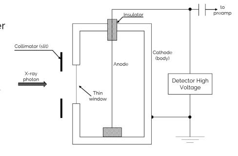
event in the first place. Wave spectrometer has two proportional counters working together to optimise count rates for all elements from Be - Pu. A flow proportional counter optimises low energy count rates while a sealed proportional counter optimises the high energy count rates.
